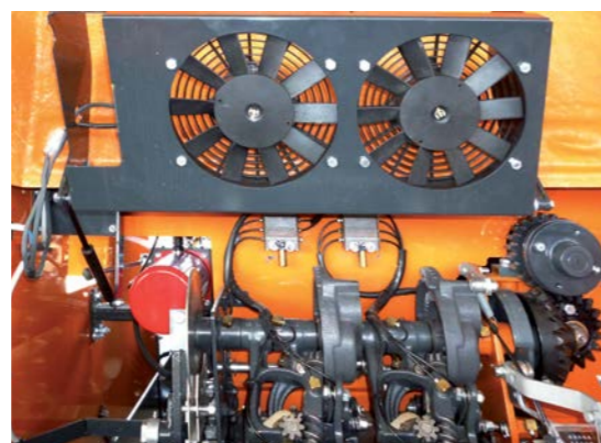
The double knotter fan, standard or optional according to baler models, allows smooth and continuous fieldwork and guarantees the durability of the knotters components.
