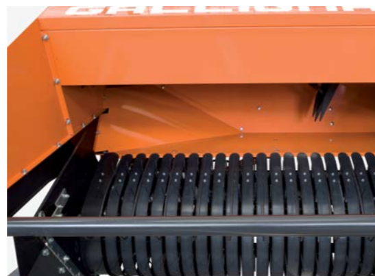
The Galignani pick-ups, always provided with cam systems to guarantee the most efficient collection of the product, can have from 4 to 6 tine bars according to the models.
