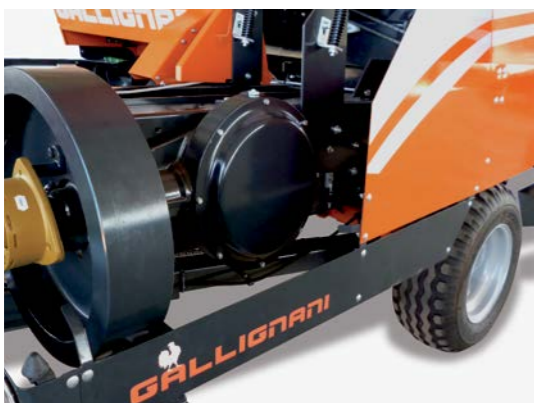
The flywheels, always of large dimensions, guarantee high performances and vibration-free fieldwork in all environments.
