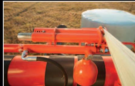
*Coupe film hydraulique (WR1100/WR1400/WR1600).*
